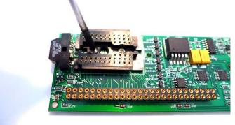
Press down on the black locating/holding pin nearest to the edge of the board
