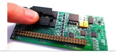
NOTE: Reattach POGO board to CPU board with care to ensure header pins are not bent. Separate instructions are available for printhead disassembly/reassembly
