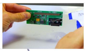
Hold the board upside-down and keep POGO connector in place with your fingers
