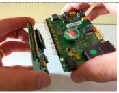
Replace the circuit board, by carefully aligning the pins and gently pressing it back into position.
