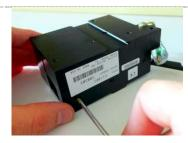
**4.** Remove the top and side casing.
