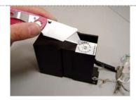
2. Unscrew the printhead side screws for the larger section of the printhead with a Phillips head (PH1) "Fine" screwdriver
