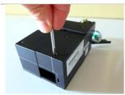
**3.** Unscrew the bottom section of the printhead with a Phillips head (PH1) "fine" screwdriver.
